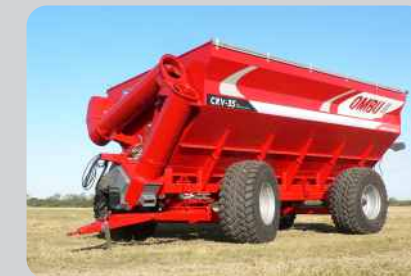
Sweeper bottom auger Two axles | Capacity: 16.5T / 35T
