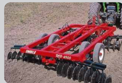
Quantity of discs: 28 to 56 Weight per disc: 72kg
