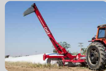
Debagger - Hydro propelled Capacity: 210T/hour
