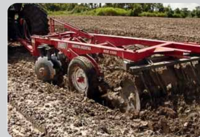
Quantity of discs: 16 to 28 Weight per disc: 65kg
