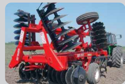
Quantity of discs: 48 to 82 Weight per disc: 104kg
