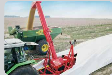
Grain Extractor - Sweeper system Capacity: 180T/hour
