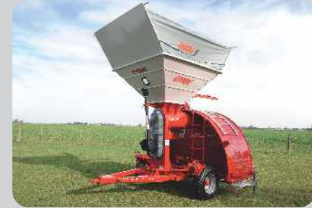
Grain bagger | 9' bag tunnel Capacity: 500T/hour
